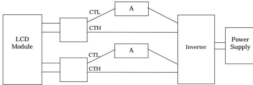
\*2) Lamp frequency of inverter may produce interference with horizontal synchronous frequency, and this may cause horizontal beat on the display. Therefore, please adjust lamp frequency, and keep inverter as far from module as possible or use electronic shielding between inverter and module to avoid the interference.
