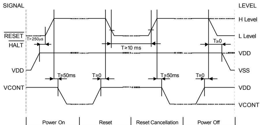
Please maintain the above sequence when turning on and off the power supply of the module.
