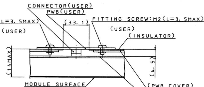
CONNECTOR (CN1) STACKING HEIGHT = 4.5 mm.
